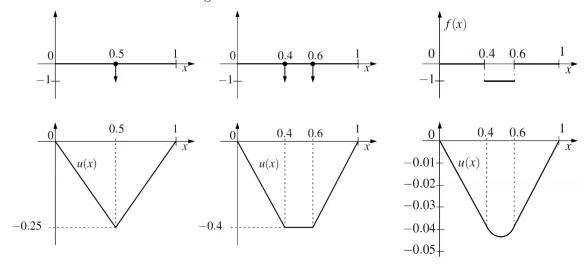
In the first case the force is all concentrated in the point 0.5, in the second case the force is distributed in the two points 0.4 and 0.6 while in the third case the force is distributed in the whole interval. In the bottom of the picture there are the solutions of the three problems. But, as you can see, the functions u(x) are not differentiable.
